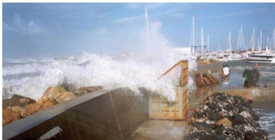
**Figure 3-5: Wave Wall Overtopping Testing in Ostia, Italy. Image courtesy of Eurotop, 2018**
